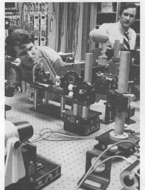
RETURN TO THE EARLY DAYS of CRF — vintage 1979 - with Larry Rahn (DMTS, 8354) and Peter Mattern (8300) in a coherent anti-Stokes Raman spectroscopy (CARS) lab. Their work of about a decade ago led to techniques that significantly increased the detection capability of CARS, which remains a primary combustion research tool today for determining flame temperatures and major species concentrations.
